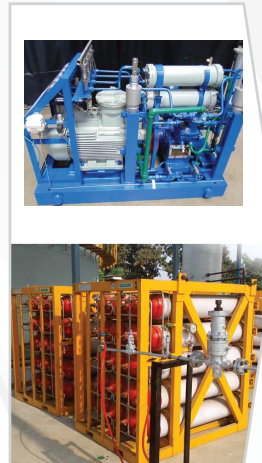
CBG Compressor & CBG Storage
