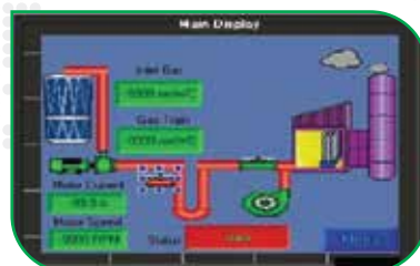
Display of Gas Train in SCADA
